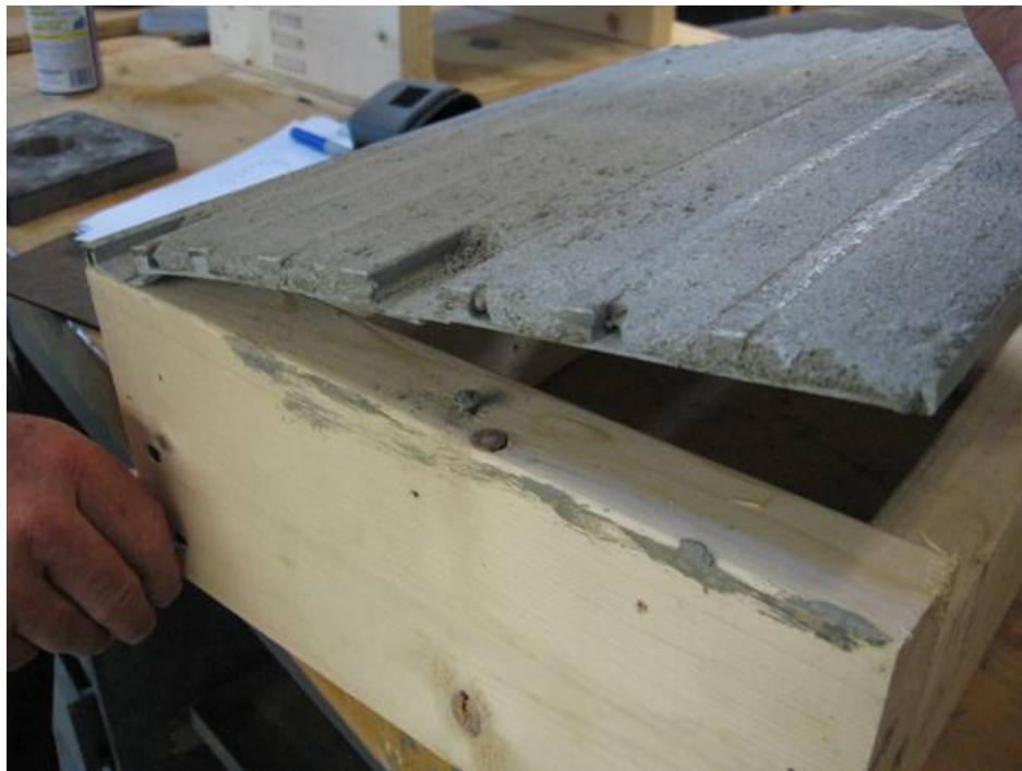
Figure 8: Local splitting of panel at screw at mid-span
