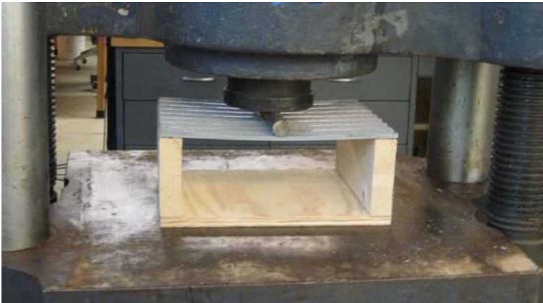
(b) Specimen under flexural load
