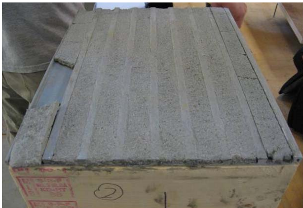
Figure 5: Concrete cracks and spalling on top surface of specimen 2
